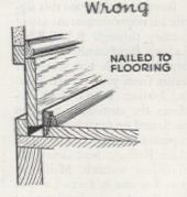
and floor should be painted or finished all the way. Then replace the molding, using 8d or rod finishing nails that go between the base and floor for a hold in the beam or underfloor. Set and putty the nails, and paint the molding. Subsequent shrinkage or expansion will not move the molding, and the base and floor can move, showing no bare wood when it comes out from under the molding.
