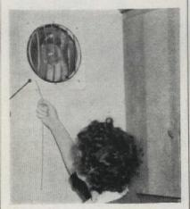
nother type of kitchen fan-one requiring no construction or special tools-can be mounted in the window. Simply lower the upper sash and slip the complete assembly into place, adjusting the sliding wings as necessary. The fan can rest on top of the sash, or be set in a little so the window can be closed in cold weather
