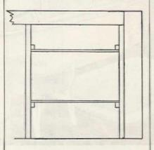
Fig. 3. A side view of the rack. Additional short uprights may be nailed to the horizontal pieces if your windows are of various sizes
