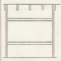
Fig. 2. This is a front view of the rack for storm sash and screens. Be careful that you measure accurately for the dividing pieces or "tracks"
