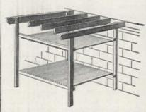
Fig. 1. This shows the completed rack for storm sash and screens. The rack is hung from the rafters making unnecessary the boring of holes into the concrete wall. Uprights are of 2" x 3" material. Horizontal members will be of 2" x 2" material
