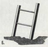
On hard, uneven ground, move top of ladder so that it rests in vertical plane. Place block under ladder leg at low spot. The drawings are exaggerated for clarity
