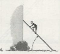
185 lbs. wt. of man and 50 lbs. wt. of ladder totals 235 lbs. Too much pressure is exerted if ladder is at 45° angle
