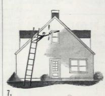
Against slanting roof, move ladder bottom to lowest part till four corners have solid contact, don't wobble
