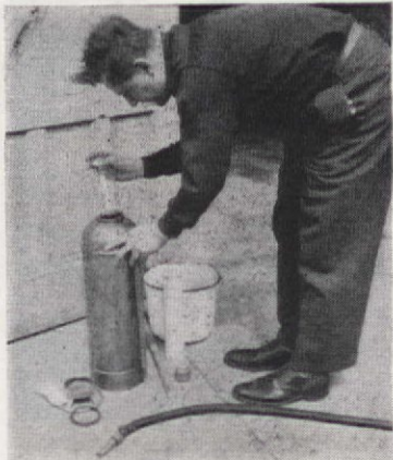
Remove acid bottle; save stopple for use in new one. Rinse shell
