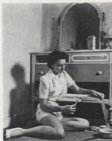
filling in all the grooves with putty so as to provide a smooth surface
