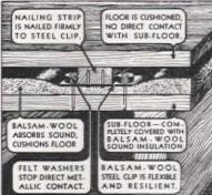
Rubber flooring in beautiful new colors and marbleized effects available for the home in thirty-six inch widths. Goodyear Rubber Co. Left: A sound deadening system for the home installed between flooring and sub-flooring consists of wool, wood strips, steel clips. Wood Conversion Co.
