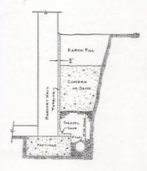
A section of a house foundation showing outside waterproofing and the location of drain tiles, and porous fill around the walls of a home
