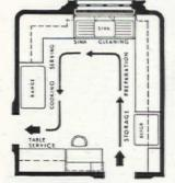
Floor-plan of the Crane Scientific Kitchen pictured above. Similar step-saving efficiency can be given to kitchens of many sizes and shapes.
