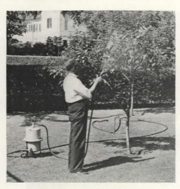
Here's a spray pump that operates on the city water pressure without manual labor. There is a rubber contraption that yields under the water pressure and so forces out the spray material. (Hydro-Air Spray)
