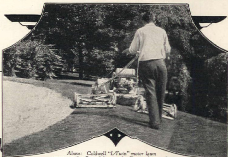
Above: Coldwell "L-Twin" motor lawn mower and roller. Mows and rolls simultaneously 4 to 6 acres a day. With gang units attached it cuts a 60-inch swath, ten acres a day.
