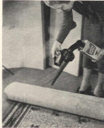
Crystals and flakes are distributed quickly and forcefully by a vacuum cleaner attachment. (Photograph Courtesy of Abraham & Straus)
