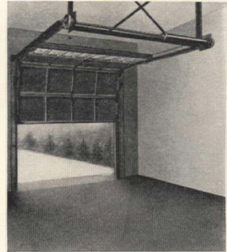
Interior view of float-over door showing special construction for minimum headroom. The door is hinged in sections. (Cornell Iron Works)
