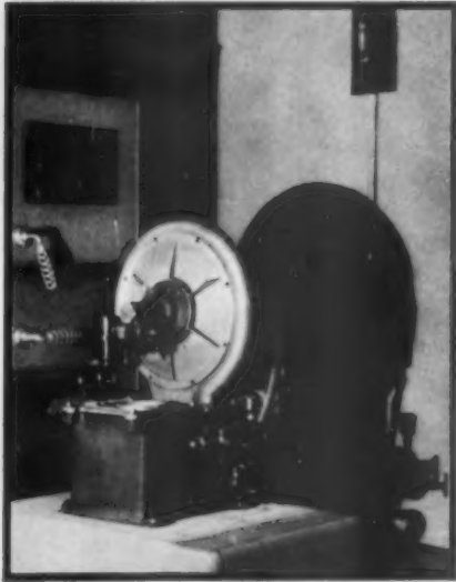
All the well-known makes of burners are dependable although their methods of operation vary considerably. The deciding factors in selecting one must be, besides price, the reliableness and accessibility of the local dealer and the type of oil available in a particular region. The burner at left will use an extremely heavy oil
