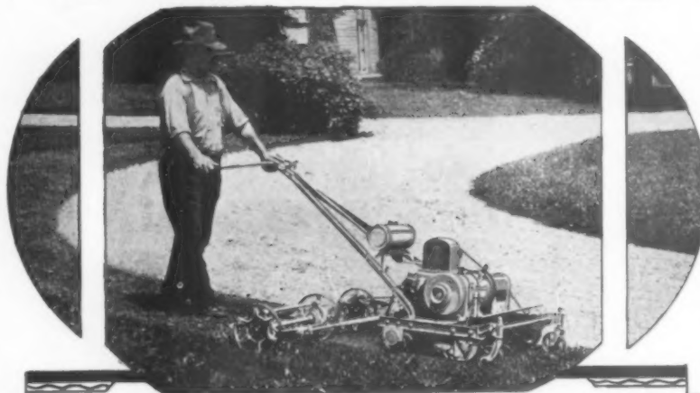
Above: Coldwell "L-Twin" Motor lawn mower and roller. Mows and rolls simultaneously 4 to 6 acres a day. With gang units attached it cuts a 60 in. swath, ten acres a day on one gallon of gasoline.
