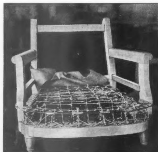
Showing how the springs should be tied many times before the upholstery is put on in a chair of good construction. This work is an art in itself
