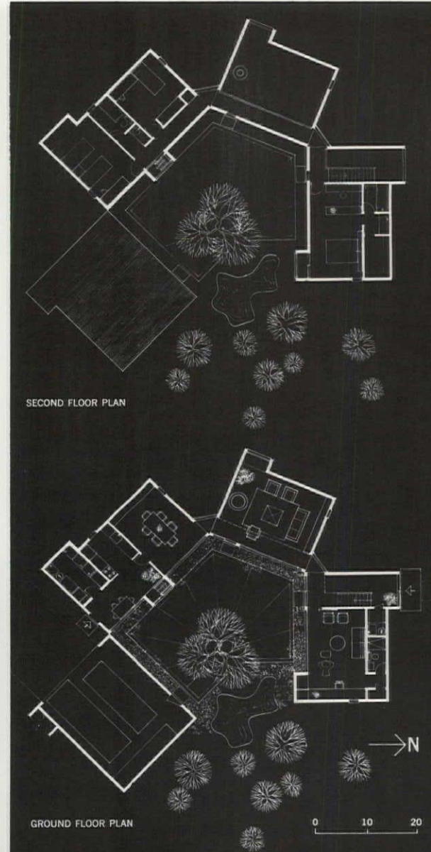
A two-story living room (left) fills the central block of the three-part house (plans above). The large glass areas of the first floor rooms face inward toward the court (right), where they are shielded from the view of passersby, as well as from direct sun.
