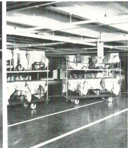
Small tractor pulls train of floats to storage. Shelving can be adjusted.
