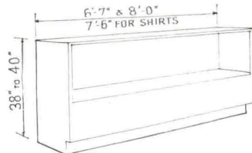
4. Display counter, used for small items and to divide clerk and customer.
