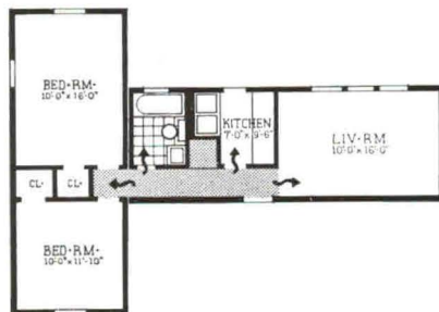
VARIOUS COMBINATIONS of three basic units, Copper Mobile Houses. Air conditioning duct is located in shaded area.
