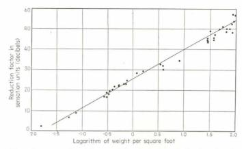
Chart showing results of Bureau of Standards Tests, indicating that the sound insulating properties of partitions tested is primarily dependent upon their weight.
