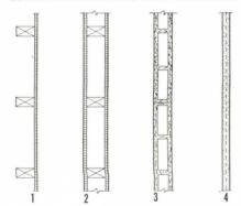
1.-2. Wood studs and wall board, unplastered, sound reduction 15 to 30 db; 3. Unplastered hollow block and light-weight masonry: 35 db; 4. Very thin solid plaster: less than 40 db.
