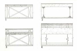
1. Regular wood joist construction, plaster ceiling, sound reduction 40 db; 2. Concrete supported by 8" open truss steel joists, plaster ceiling: 55db;
