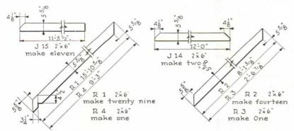
To the power-saw operator go typewritten instructions (see above) as well as this lumber detail chart. From such drawings the workman sees the angle of saw cut required. The framing members are detailed to a 1 in. scale.
