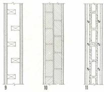
9. Staggered studs, 3-coat plaster on plaster board, sound reduction more than 50 db; 10. 8" brick, plastered: 55 db; 11. Hollow block, plaster on resilient furring; just under 60 db.
