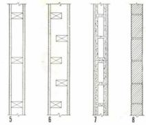
5. Wood studs, praster on lath, sound reduction over 40 db; 6. Same with staggered studs: 45 db; 7. Hollow block, plastered: 45 db; 8. Brick, 4 in., unplastered: 45 db.
