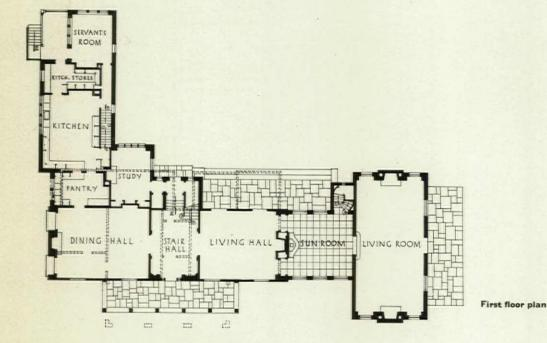
The original house was well built and structurally sound, but of a nondescript type, out of character with the architecture of the district, and inadequate for the needs of the owner. The alteration consisted of encasing the existing house with clapboards, tearing off the overhanging cornices, and adding kitchen and living room wings. The interior of the house was
