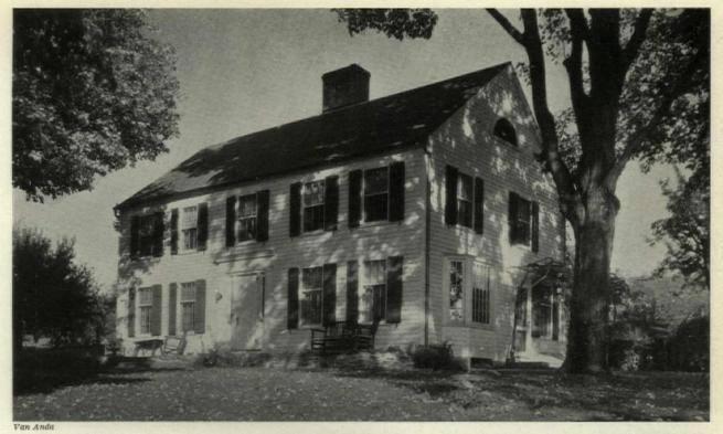
The stairs were relocated in an entry hall corresponding with the former living room, two baths were installed upstairs. The addition consisted of a wing having a single room for living on the first floor and two new bedrooms on the upper floor. Note the effect of removing the front gable and the projecting eaves. Total cost of operations \$10,000.
