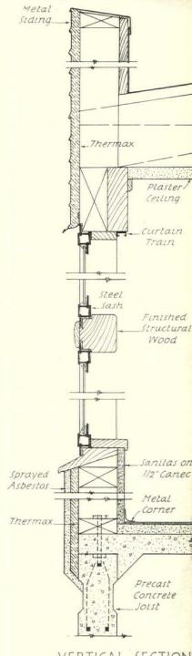
VERTICAL SECTION (Wood Chassis Construction) Scale 14/2"=1-0"
