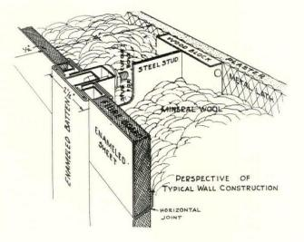
Top, bolting together the prefabricated steel frame and placing first floor joists. Center, bridging the light-weight truss joists of the first floor. Bottom, construction details showing form of steel stud, exterior enameled panels and batten, as well as the mineral wool insulation
