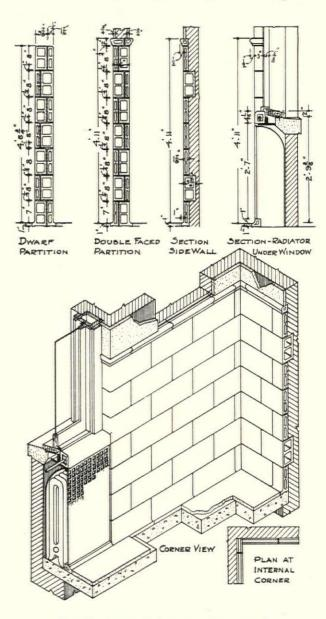
Details of construction of sanitary glazed terra cotta interior walls and partitions
