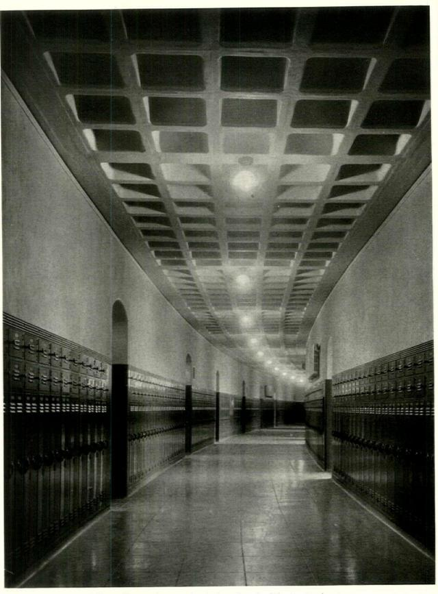
Ceiling coffers are the natural and planned result of the structural system which employs pan forms for the concrete. Light gray walls contrast with the purple-maroon of the locker rows. The floor is rich Pompeiian red
