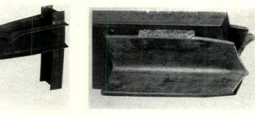
Tests showing strength of welded joints. Above, tension test specimens of fillet welding. At left, flexure test under concentrated load, no weld failure; and parallel shear test, no weld failure
