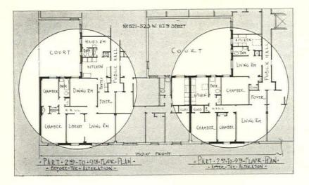
A plan study by Manoug Exerjian, architect, which illustrates graphically the possible revision of a large suite, cumbersome and unrentable, into two small modern apartments. Note particularly the manner in which the existing soil and water lines have been utilized in the new layout
