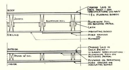
Details of floor and wall system using aluminum foil as insulation and canvas as finish material. Developed by Kocher & Frey, architects
