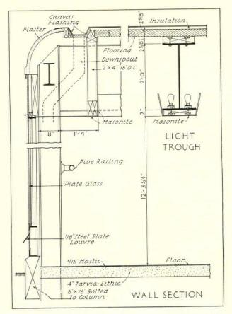
A section through the semicircular, glass walled exhibition space showing its simple but efficient construction. The light trough is especially noteworthy, ingeniously using the structural beam as an integral part of the effective indirect lighting system
