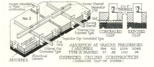
Details of a system for installing furred ceilings of incombustible acoustic tile
