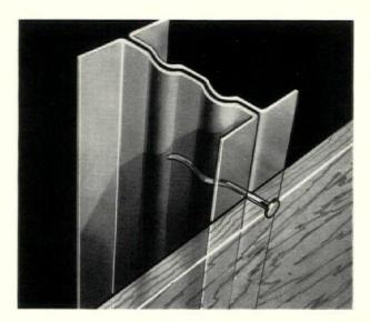
Top, carpenters nailing insulation board to steel studs. Center, portion of framing, showing platform-type construction, stair opening, plumbing stacks, joist hangers and reinforcing for concrete floor slab. Bottom, 3/4-in. board being nailed to Stran-Steel stud
