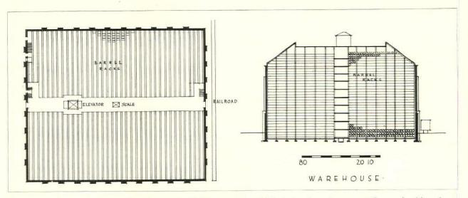
Plan and section of bonded warehouse at Hiram Walker plant, in which during the aging process thousands of barrels are stored on heavy timber racks, built as detailed below, to prevent damage to the barrels and to avoid condensation
