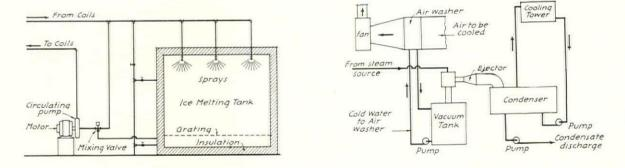
Schematic diagram of central cooling system, left, using ice as the refrigerant. The cooled water is piped to the coils over which the circulated air is blown. Right, general arrangement of a steam ejector cooling system
