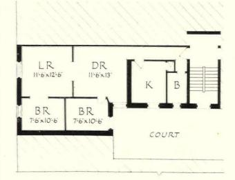
Plan of typical present-day Bronx apartments, inconvenient in plan, with most of the rooms facing on walls only a few feet away
