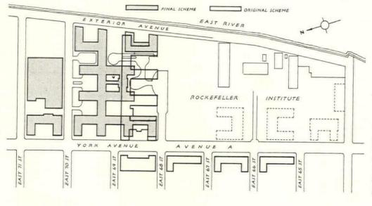
The gray block indicates the final form of the plan for the buildings as constructed. The dark outlined blocks indicate the buildings as first planned before the property to the north of the original site was acquired. The elimination of the street running through the property made possible the unified plan
