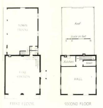
In keeping with the general architectural character of other public buildings in the community, this fire station represents a successful solution of the often recurring problem of supplying a distinguished building at a minimum cost. Built of brick, with shingle roof and white painted wood trim, its plan is simple and yet adequate
