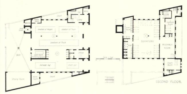
The flexible California style is here happily adapted to a small fire station. It is of fireproof construction, with walls of common brick and stucco exterior. The roof is of Granada tile laid in white mortar. Doors and windows are wood
