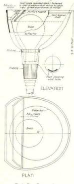
Details of new type efficiency floor lamp
