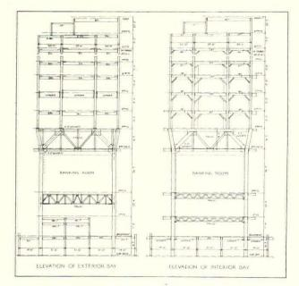
Typical framing diagrams showing the trusses and knee-braces
