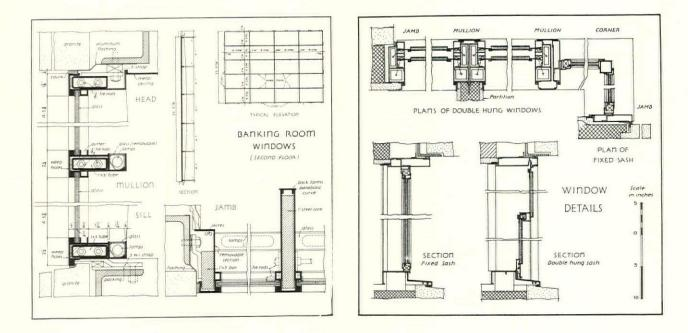
Aluminum was used for most of the windows throughout the building, due to its color, its light weight, its comparative resistance to corrosive stain. These details show the result of designing for a minimum thickness in structural members. This is particularly noteworthy in the case of the banking room windows where mullions are only 1 in. thick
