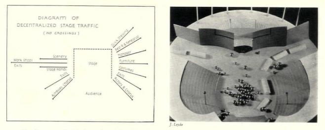
The diagram at the left shows the relationships of the services or functions to the stage, and at the right illustration of the model showing use of arena for pageantry, indicating the entrance and egress for actors, floats, etc.
