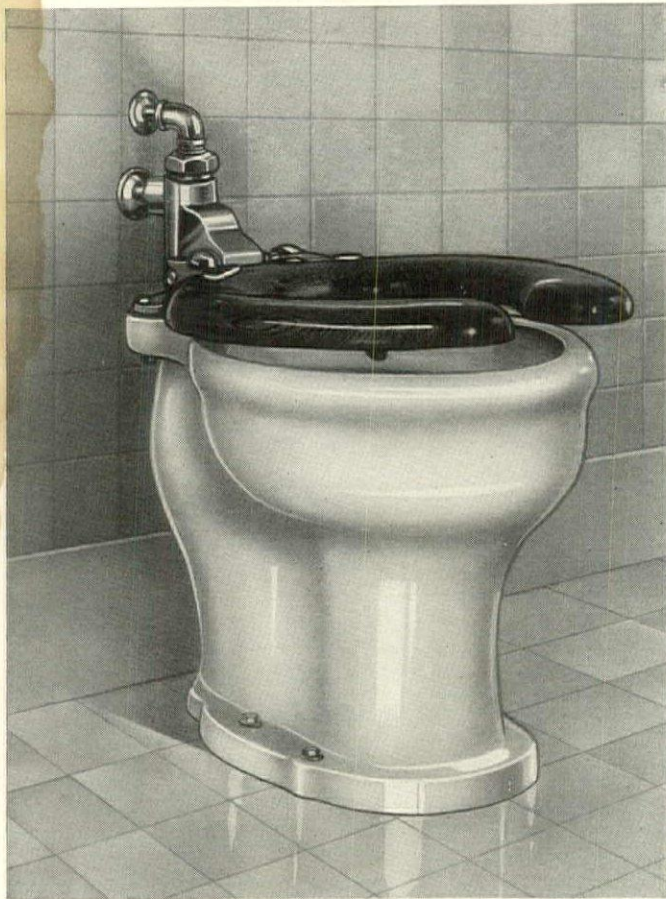
Vogel Number Ten-A Seat-Action Closet with syphon jet bowl. Tank is in the wall. Flushes on air and water pressure.
