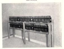
THIS PHOTOGRAPH SHOWS the 60-cell Exide Battery that supplies the Hilles Laboratory with current for experiments.
