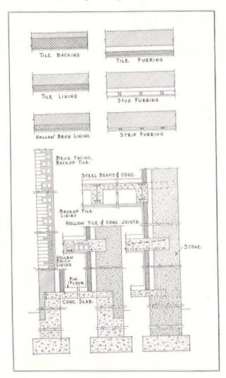
Diagram Showing Various Types of Masonry Wall Construction. Brick Facing is Shown with Various Types of Backing and Furring. Several Floor Types are Also Shown
