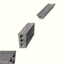
SPEED in construction, independent of temperature, is a highly valuable feature of Natco Flat Arch Floor. Centering is hung; no nails are used. Centers need remain in place but one-tenth to one-fourth the time required under other forms of construction. Floors beneath are accessible for work by other trades. The all-tile ceiling requires only two coats of plaster. Holes may be left, or cut at any time to accommodate pipe work and later easily patched.
