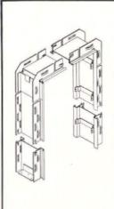
The Kalman Steel Buck, which replaces wood buck, ground and standing trim. Doorways are simplified and beautified in appearance. Net wall space is increased. Strength is added. Write for file folder giving 15 advantages of Steel Buck, and Jamb and Buck.
