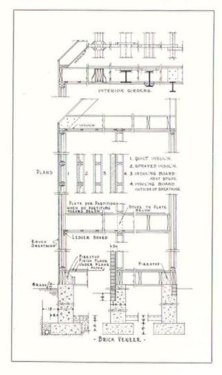
In using brick or stone veneer on frame, there is no particular advantage in leaving an air space between the veneer and the supporting frame wall. Such an air space only serves to complicate and increase the cost of window construction and makes it more difficult to prevent wind and water entering between the frame and veneer. Only working space for the veneer is required.
