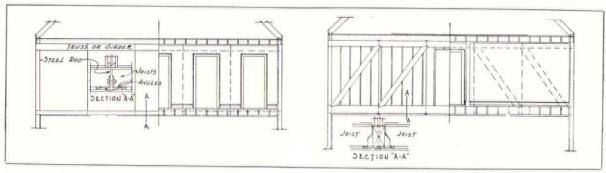
Two Methods of Supporting a Second Story Over a Long Span
