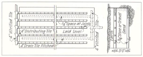
Subsurface Sand Filters are Built When the Ground is to be Planted for Use. Dimensions Proportioned to the Volume of Effluent to be Filtered
