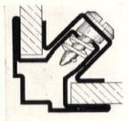
Sash B-1 and Corner Bar B-2 of "B" construction (Full Size). Sufficiently sturdy and graceful for the largest and finest store fronts. .
