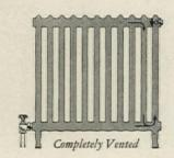
IN-AIRIDS located within the radiator cannot be tampered with. Their invisibility also adds to the appearance of the radiator.
