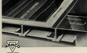
Rigideck—the new Armco Ingot Iron Roofdeck is as easily laid as board. Its interlocking ribs occurring every six inches are securely attached to the purlins, providing a rigid, smooth, unperforated roof deck adapted to all buildings. Weight of completed roof approximately 5 pounds per sq. ft. Fireproof and economical.
