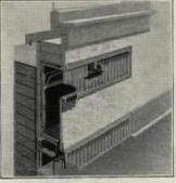
Sectional view of complete Trane Concealed Heater installation
