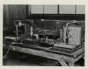
Apparatus for Testing Heat Conductivity of Building Material by Hot Plate Method
