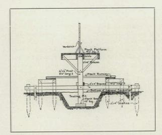
Fig. 9. Platform for Testing Bearing Capacity of Soil
