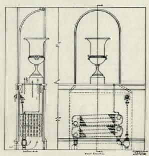
Method of installation showing inlet opening from the reverse wall.
