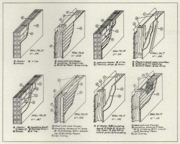
Fig. 1. Common Types of Wall Construction. The Smaller the Numerical Value of "U," the Coefficient of Heat Conductivity, the Better the Wall as an Insulator
