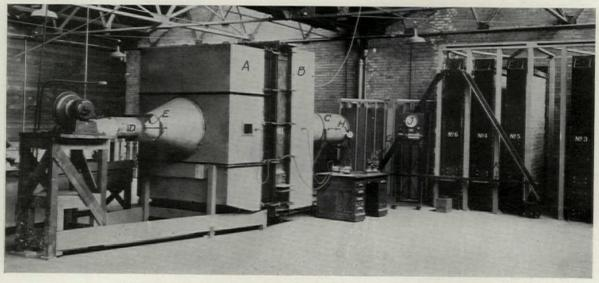
Testing Equipment for Determining Air Flow Through Brick Walls. Several Test Panels Are Shown at Right
