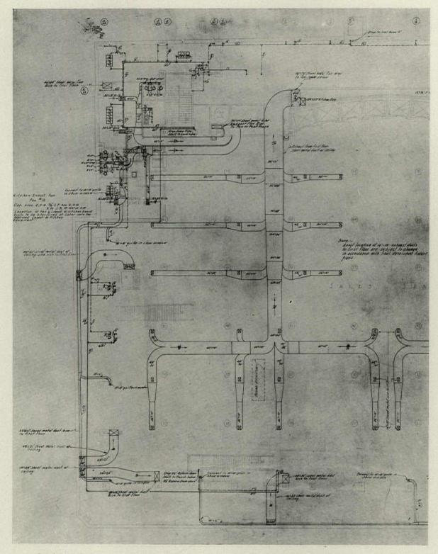
One-half Plan of the First Floor of the Davison, Paxon Co. Department Store, Atlanta, Showing the Heating and Ventilating Layout
