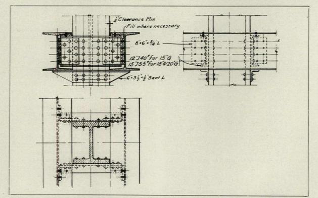
Details of Typical Connections for Cantilever Construction Shown in the Plan at Top of Page. Seat Angles Are Not Designed to Carry the Load, Which Is Supported by Channel Diaphragms
