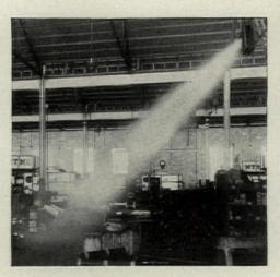
5 Seconds Afterward the heat is down to the floor and starting to spread.
