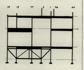
Fig. 3. The alterations in the structural frame shown here were to accommodate the new shop front shown on the preceding page
