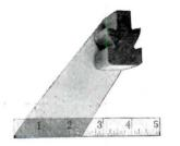
NOTICE THE DIFFERENCE in the amount of shadow cast by the steel Lutton Solar V-Bar (right) in comparison with the ordinary wooden bar (left). This difference, when totalled over the whole greenhouses, actually affects the yearly production of flowers.
