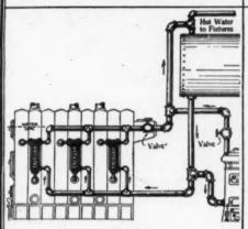
Battery of Excelso Water Heaters Connected Up for Larger Requirements The Excelso Water Heaters are shown cross connected with coal water heater so that either or both may be used
