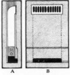
(A) Cross section view of Trane Heat Cabinet as installed in the wall. Air inlet and heating element at bottom, air outlet at top. (B) Front view of the finished installation. Only the inlet and outlet are visible. Dotted lines indicate position of Cabinet in the wall.
