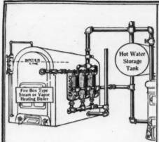
Battery of Excelso Water Heaters Connected to Steel Type Heating Boiler Typical installation for large apartment houses and other larger types of buildings where large amounts of hot water are required
