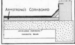
Typical method of insulating a concrete-slab roof-deck.
