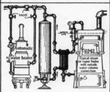
Excelso Water Heater Cross Connected with an Automatic Gas Water Heater Gas heater for summer use; Excelso Water Heater for winter use
