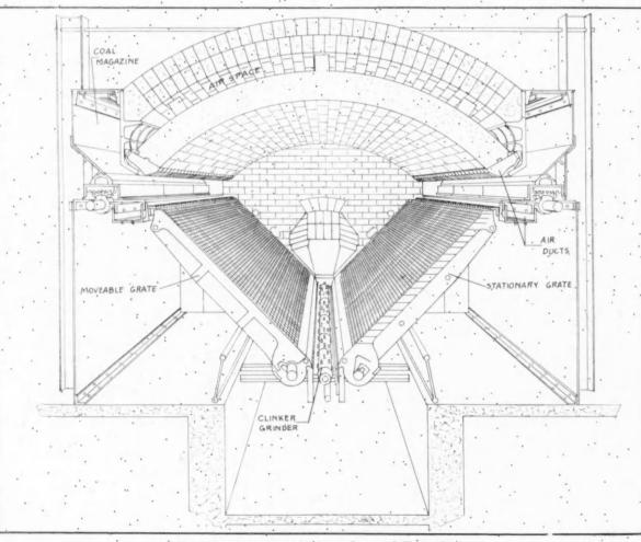
Fig. 49. Side Over-feed or Opposed Type Stoker
