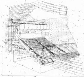
Fig: 42. Hand-driven Mechanical Stoker
