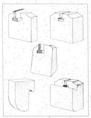
Fig. 46. Special Blocks for Flat-arch Construction
