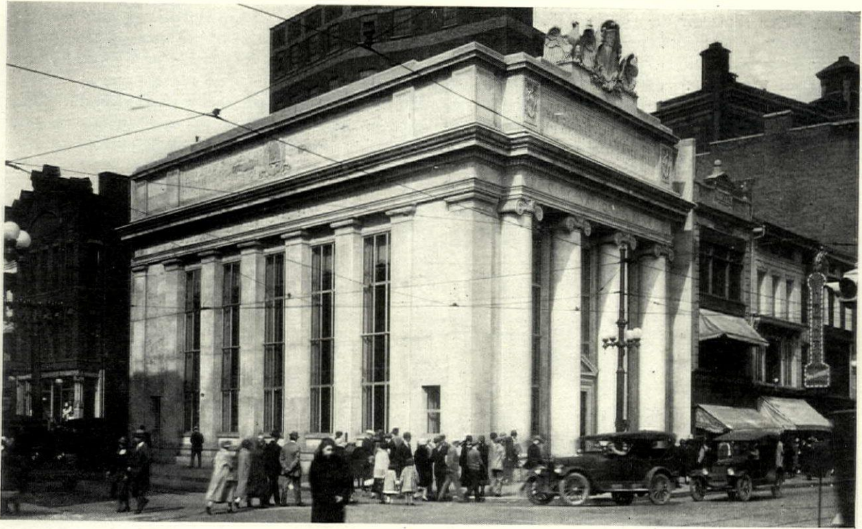
High Attic Walls Provide Space for Lettering. City National Bank, Binghamton, N. Y. Alfred Hopkins, Architect
