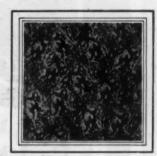
4. This striking effect can be secured by applying a light color as a finishing coat, over a ground of a darker color. Write us if you would like samples of the mottled effect.
