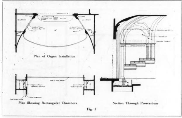
ium arch, with a deflector outside of the organ chamber to deflect the tone down in the direction of the orchestra pit. This tends to make the tone spread under the balcony, giving excellent results, since the tone fills the entire house. See Fig. II.
