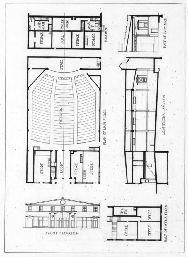
Elevation, Longitudinal Section, and Plans of the Basement, Main and Mezzanine Floors of a Motion Picture Theater for a Small Town J. H. Phillips, Architect
