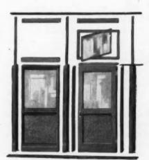
The units of Telesco Partition are standard and interchangeable. Fastened entirely with screws.
