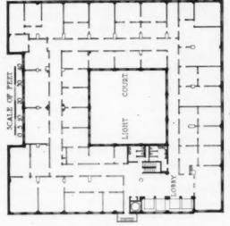
Typical Floor Plan Showing Possible Office Arrangement
