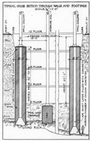
Cross Section Through Substructure, Barclay-Vesey Telephone Building
