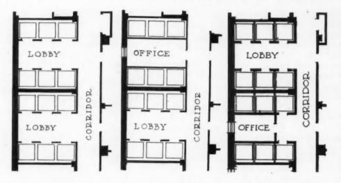
Express and Local Elevators Arranged in the Same Batteries. Floor Area Between Express Elevators Used for Office Purposes. Straus Building, Chicago
