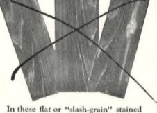
In these flat or "slash-grain" stained shingles, the hard, flint-like surface of the flat grain cannot absorb and hold stain.
