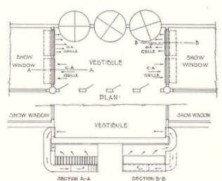
Fig. 2. Arrangement of Radiators and Doors
