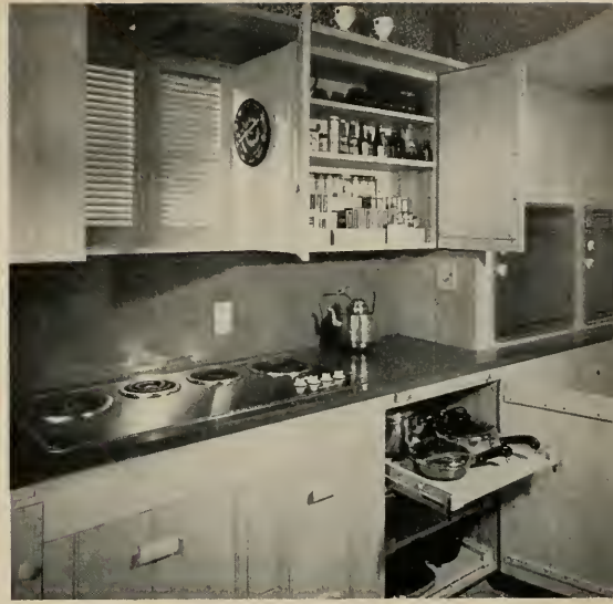
COMPACTNESS is keynote of this kitchen in home of Milton Faland, designed by Richard Sundeleaf—note stacked utensil storage and stairstep spice shelves as outstanding examples of compact planning.
