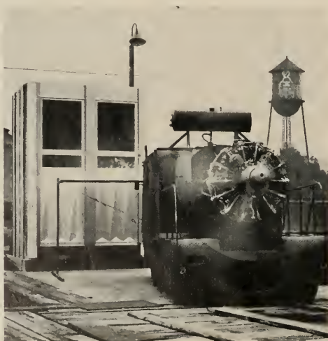
LIC Typical Mock-Up for testing weather-tightness and deflection of curtain walls prior to installation on buildings.
