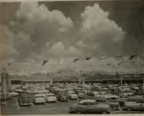
TYPICAL PARKING AREA during shopping period. Angle parking with stores of 55 degree prevails; extra wide stall spaces permit ease of entering and exiting from cars.
