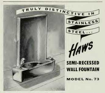
Smartly designed, extraordinarily convenient is this entirely new HAWS Semi-recessed Fountain that takes up little space in corridor or room and has drinking fountain head and operating lever handle accessibly located opposite one another on the top platform. An access panel in wall is NOT required for this fountain and all fittings are accessible from under bowl.
