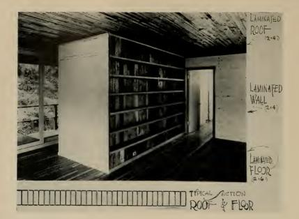
with adhesives which provide an everlasting bond are able to withstand terrific wind pressures and excessive amounts of strain and stress imposed by undulations and gyrations of earthquakes. Glued laminated walls and floors are very fire-resistant. Laminated solid wood keeps its strength unimpaired thru fires of considerable duration. (Test this in your own fireplace by burning a solid book, and then some loose pages).
