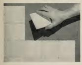
Described as the most important development in twenty years of tile making, Mikro-sized tile differs from standard tile in that it has spacing lugs on two ad-jacent edges only. These lugs are twice the size of regular lugs, thus providing standard 3/64 in. joints. The other two edges of the new tile are precision ground, assuring absolute uniformity of size.
