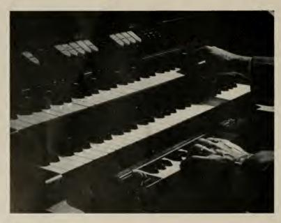
Lower two-octave keyboard is that of the carillon, rigidly mounted to organ console.
