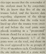
used to lift the bundles of joists to the roof, the crane operator would have been relying upon signals from a man on the roof to determine when to release the weight of his bundle on the roof system. A slight error could have resulted in dropping the load onto a pair of trusses, thus precipitating the failure.
