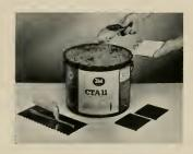
The development results from a new ceramic tile adhesive; tan colored, synthetic rubber, ready for use when taken from container. By using notched trowel, coverage is 60 to 70 sq. ft. per gal., and 1 lb. of adhesive will do the work of 40 lbs. of wet mortar.
