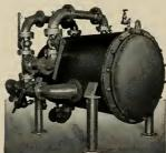
Operating engineers report that daily laboratory tests show this filter will completely remove suspended matter either colloidal or solid, bacteria 80% to 100% depending upon type of bacteria and grade of diatomite used. Thus reducing the required chlorination to a very low point. Sizes vary Irom 25 sq. ft. to 100 sq. ft. of filtering surface; flow capacities over  $2\frac{1}{2}\text{M}/\text{G}/\text{D}$  per unit.
