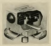
Designed for use with electric motors and gasoline engines, the VAC-ON switch has many uses as a circuit-breaker or control, and also serves as a warning control where operating conditions depend on a vacuum. Switch is mounted on the suction line and wired to power supply—when suction falls below a predetermined pressure switch automatically cuts off motor or enaine.
