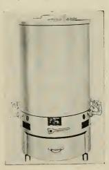
It uses LP, manufactured, natural or mixed gases at a rate of 50,000 BTU per hour input. Standard unit has ¼" thick steel plate combustion chamber and also furnished with heavy refractory lining at extra cost. Solves problem of hospitals, clinics, restaurants, stores, motels and institutions. Manufactured by Incineration Division, Bowser, Inc., Cairo, III.
