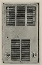
Equipped with built-in thermostat, pressure type fan with long life ball bearing motor, the heater is available in 2, 3, 4 and 5 kw. for 236-volt a.c. operation. It is finished in smooth silver gray hammertone, or in neutral prime coat.
