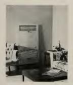
The heater is available with inputs of 37,000 BTU and 45,000 BTU for natural or manufactured gas; require a wall opening of only 28" by 51"; finished in baked enamel; and top panel louvers give a downward and outward direction to the warmed air flow, while lower louvers near the base (which is raised off floor) give off radiant heat.
