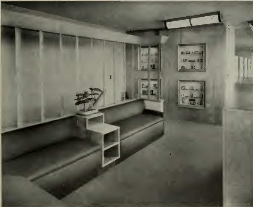
BELOW —A section of the Store where show cases have individual show-case illumination. Finished in natural Maple. Prefabricated booths in the adjacent Beauty Salon have a 2-inch thick, smooth finish, masonite wall.
