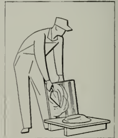
2. Mortar is applied to wall and Ceramic Veneer back.
