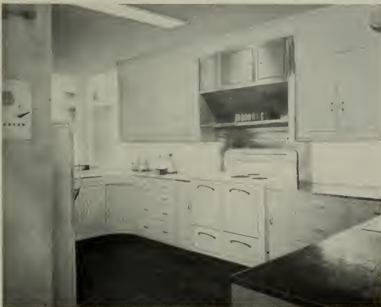
LEFT —The kitchen has general lighting provided by a recessed fluorescent troffer unit. The range is pinhole spotlighted. Daylight is admitted through glass block panels concealed beneath the cabinets. Many other ultra modern items are included.
