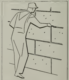
4. Joints are pointed. Surface is washed as last step.
