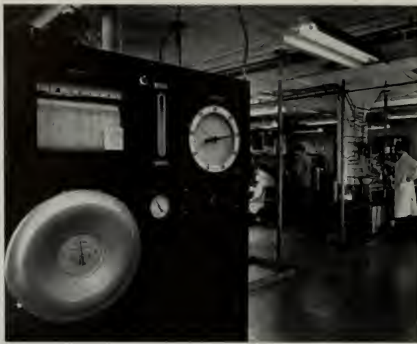
View of organic research laboratory, one of the many specialized centers within the Pabco Research Building. Shown on left is instrument panel of equipment for studying the processing of asphalt and pitch.
