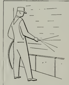
1. Structural wall is wet; Ceramic Veneer soaked.
