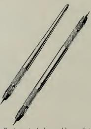
Features include a rubber collet in neck of chuck which grips lead and "cushions" against undue pressure. The hardened steel chuck cannot be damaged when sharpening leads against file or sandpaper. Uses all standard drawing leads.
