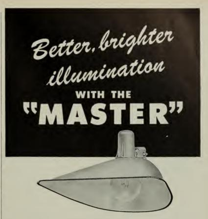
A highly efficient floodlight for use in service stations, parking lots, yards and other areas where maximum spread of light is desired. Finished in porcelain enamel, with neutral gray exterior. Supplied with mountings for wood cross-arms, l'' to  $l\frac{1}{2}''$  pipe cross-arm or slip-over  $l\frac{1}{2}''$  pipe mast. Takes 750/1000/1500 W. lamp.
