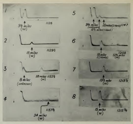
Copy of original British photographic radar record made on a cathode ray tube trace. The time of each photographic exposure is given on the right-hand side. The "techo" caused by a Wallace aircraft (W) on its outward journey is clearly visible (at increasing distances) in 1 to 4, and on its return journey (at decreasing distances) in 6 to 8. Nas, 5 and 6 indicate a farmation of three Hawker Hart aircraft which came into the radar view uninvited.
