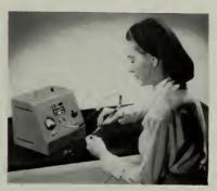
A pair of insulated forged copper tweezers are connected with the unit which is operated with a foot switch.
