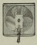
Set on window sill, attached by two screws to jam, driven by capacitor motor. Blades are of sheet aluminum. Dimension  $29 \times 9 \times 24$  inches.
