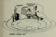
The cylindrical damper is raised or lowered by turning the extended shank of the operating screw. Any air volume may thus be quickly and easily obtained. Complete handbook available by writing manufacturer.
