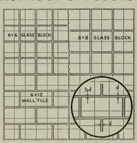
THE MORTAR JOINT is automatically provided for with modularcoordinated units. Net size plus standard mortar joint {d} equals nominal size, thus the architect need work only with nominal dimensions.
