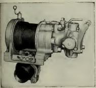
Capable of lifting 500 lbs., the "AIR WINCH" AW-80 weighs only 85 pounds, has a rope capacity of 150 feet of ¼-in. rope, is 18 inches long, 9½ inches high and 11 inches wide. It is powered with a fourcylinder, reversible, piston type air motor. Can be mounted in any position. Complete information Bulletin No. 76-H.
