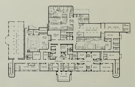
GROUND FLOOR PLAN—Showing unique location of surgery and accessories including anesthesia, fracture, supply, work space; and storage, heating plant, laundry and kitchen.
