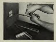
It is a triple-purpose screw driver tool with a "power-arm" arrangement that gives extra power for unlocking rusted screws, or may be used as an ordinary screwdriver by folding the "power arm" into the handle.
