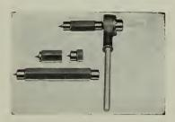
The compact head allows centering of holes within 11/4 inch of the nearest obstruction. Any standard wood bit can be used and steel drills can be used with an adapter chuck.
