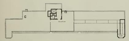
ROOF PLAN—Containing Solarium, and also designed for use as a helicopter landing for the future.
