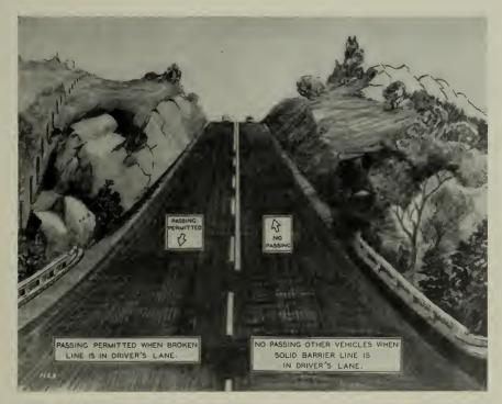
"NO PASSING" Yellow Line Doomed: The YELLOW traffic line on California's State highways is being replaced by the uniform National system of highway signs and traffic control devices—two continuous parallel white lines where passing a vehile is prohibited, and a combination solid white line where passing is permitted IF the broken line is in the driver's lane.
