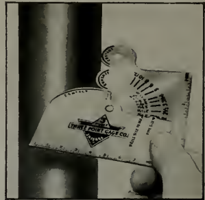
Convenient pocket-size gage for pipe measurement.
