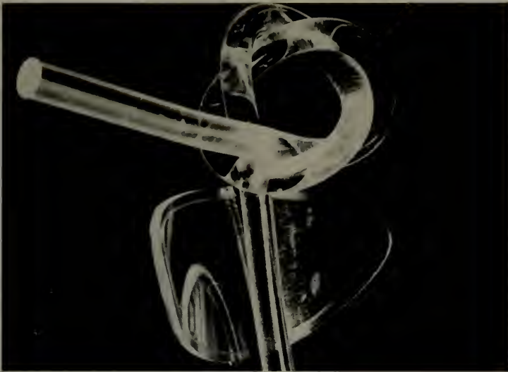
A light shone at one end of this snaky rod of "Lucite" methyl methacrylate resin—travels to and out the other end without heating the crystal-clear plastic. Ability to "pipe cold light around curves" makes the material particularly adaptable to medical instruments. A plastic gas mask lens is shown with the bent rod.
