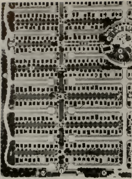
Detail of Mr. Troedssen's plan of "Sofetown," showing new dead-end streets, old streets converted to park areas, part of one of the community centers, and the insulating strip of park around the perimeter. Garages have been turned around and immediately adjoin the new access streets.
