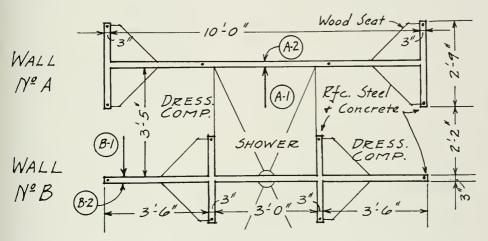
Plan of unit, consisting of shower and dressing compartments, tested for structure and seismic resistance at Kraftile plant, Niles. Point of test in Wall A is indicated by circled "A-I" and in Wall B by circled "B-I." Units were designed for Girls' Gymnasium in Vallejo High School by John J. Donovan, Architect, As developed at Kraftile plant, structure is of terra cotta wall units reinforced into a monolith.
