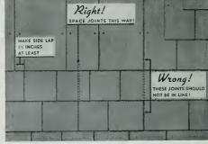
THE CORRECT SIDE LAP AND PROPER BREAKING OF JOINTS IS IMPORTANT, BUT EASILY ACCOMPLISHED
