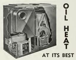
...is presented in the H. C. LITTLE FULLY AUTOMATIC FURNACE BURNER UNIT — highest quality engineering and construction — exclusive "Hear Trap" all steel welded unit — clean filtered and humidified air — constant automatic temperature control — quiet, economical operation, burns low-priced furnace oil — output 120,000 BTU per hour. Also made in smaller sizes for small homes and commercial installations. Over 50,000 H. C. Little Units in service.
