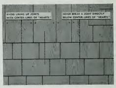
FLAT GRAIN SHINGLES IN GRADES NO. 2 AND NO. 3 SHOULD BE PROPERLY APPLIED AS SHOWN ABOVE
