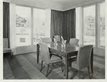
Picture windows lend out-of-door atmosphere to this room which overlooks flower covered terrace. The windows are aklo plate, a heat-absorbing glass that reduces sun-ray heat and minimizes glare.
