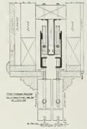
Joins with a 3¾" stud wall . . . steel studs . . . adjustable steel and wood track. Can be used for screen doors in connection with French doors. Send for detail drawing.
