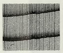
CROSS SECTION OF RED CEDAR SHINGLE SHOWING AIR-FILLED HEAT INSULATING CELLS—THERE ARE SEVERAL MILLION IN EVERY CUBIC INCH OF WESTERN RED CEDAR WOOD, DARK HORIZONTAL LINES ARE WOOD RAYS THAT REINFORCE AGAINST SPLITTING, VERTICAL DARK LINES MARK THE LIMITS OF ONE ANNUAL RING, MAGNIFIED 40 TIMES
