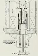
Joins with a 3½" stud wall . . . steel studs . . . adjustable steel and wood track. Can be used for screen doors in connection with French doors. Send tor detail drawing.
