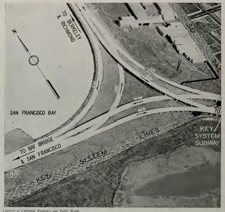
"N"—North twin structure. "S"—South twin structure. "A"—Southerly branch of East Shore Highway. "B"—Central branch approach. "C"—Northerly branch of East Shore Highway. "M"—Mole or main line approach. "AN"-Travel from "A" line to north structure. "SA"-Travel from south structure to "A" line. "SB"-Travel
