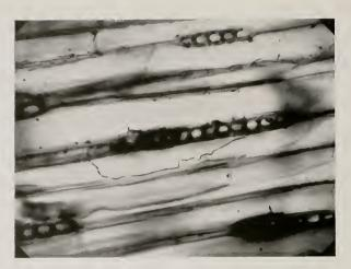
Fig. 4—Photomierograph showing minute fungous hyphae in the wood of the wall of a gallery of the dry-wood termite (Kalotermes minor). Section from the rough surface of gallery in the apparently sound, dry wood of a Port Orford cedar pole.
