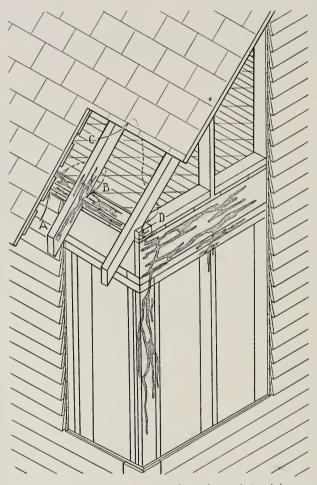
Fig. 10—Diagrammatic sketch showing workings of two colonies of the common dry-wood termite, Kalotermes minor, based on numerous observations of colonies in houses. The lines AB and CD mark the assumed original routes of entry of the two colonizing pairs. The galleries of the two colonies are not connected with each other.
