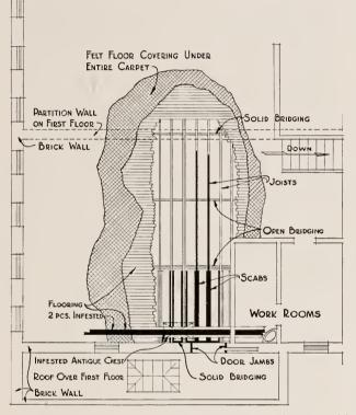
Fig. 14-Plan of building attacked by the dry-wood termite, showing in solid black the location and extent of infestation.
