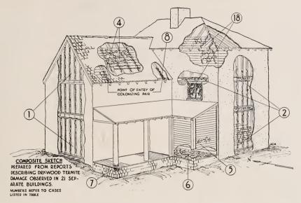
Fig. 19-Illustrating points of attack in buildings by the dry-wood termites.
