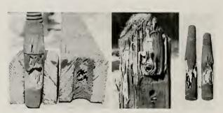
Fig. 18—Further examples of damage to pole shown in Fig. 17. (a) cross-sections of the crossarm with one pin in place. (b) Top of pole partly dissected. (c) Two of the four infested pins.
