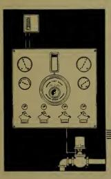
Day and Night Thermostats, Clocks, and Switches may be arranged in a wide variety of combinations for the control of branch heating mains serving various sections of the building. Differential thermostats are available to maintain proper relationship between out-door and radiator temperatures.
