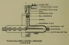
DIAPHRAGM OF BOILER INSTALLATION
