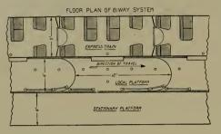
Driving motors are stationary beneath the tracks at intervals of about 1,000 feet. This greatly reduces another operating noise. Running lengthwise beneath each train is a "T" section, the flange of which runs between driving wheels of the motors. Operation of the entire system is so timed that the stopping and transfer intervals are positive and automatic. Error is impossible.
