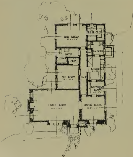
PLAN, STANLEY WILLIAMS HOUSE, LOS ANGELES Henry C. Newton and Robert D. Murray, Architects
