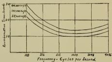
Fig. 1-Optimal reverberation characteristics for rooms of different size which are to be used for both speak-
