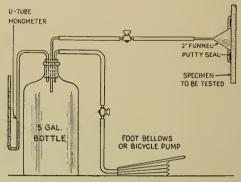
Fig. 2—Arrangement of apparatus for determining the porousity of acoustical plaster.
